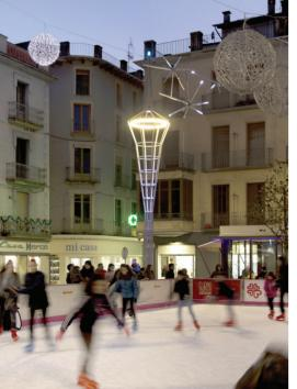
FRAMEWORK The tube structure minimises the visual impact of the columns while, at the same time, capturing and reflecting the light from the luminaires, turning each column into one large lamp.
