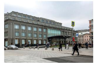
A pedestrian crossing is underlined by paving in order to indicate the pedestrian priority over cars. It also refers to the history of the street denoting a bridge over the river. The pedestrian crossings are also equipped with a system of steel tactile indicators simplifying navigation for blind and visually impaired.
